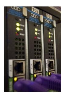
Amulet Hotkey DX Rack KVM Extenders and DXZ zero clients use Teradici PCoIP processors to provide anywhere access to graphics, media systems and tools without loading the workstation CPUs or impacting the operator experience. Media systems and workstations are centralized in the data center and compact DXZ zero clients are used in the MCR to connect to any system.
